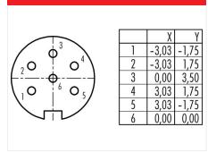
Contact arrangement (Plug-in side)
